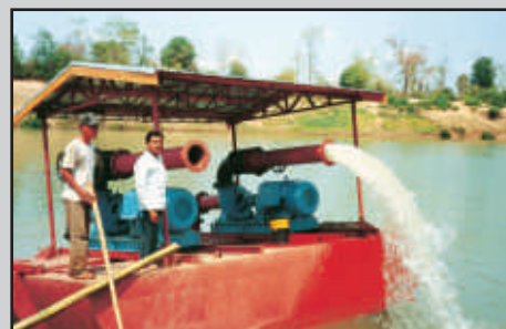
Pontoon mounted pumps for irrigating paddy fields along Mekong river, Lao PDR
